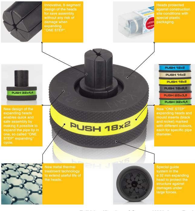
Full identification of System KAN-therm Push diameters for more convenient assembly.
