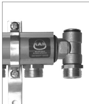
Manifold 71A and 75A upper beam with extension consisting of tee connection (R542), cap G \frac{1}{2} " (6095.34) and nipple G \frac{1}{2} "xG \frac{3}{4} " (P05).
