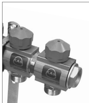
Manifold 71A and 75A upper beam with extension equipped with actuator valve (712) and cap G1" (6096.43). The element connected to the manifold by means of nipple G1" with special seal (R543).
